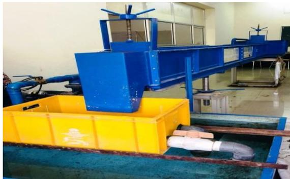
*Fig.2 Tilting Flume*
