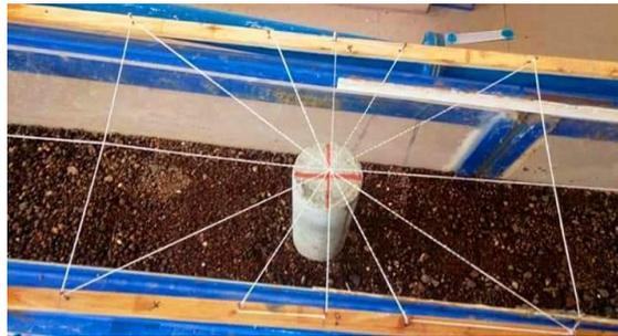
*Fig.1 Arrangement of Pier in Tilting Flume*
